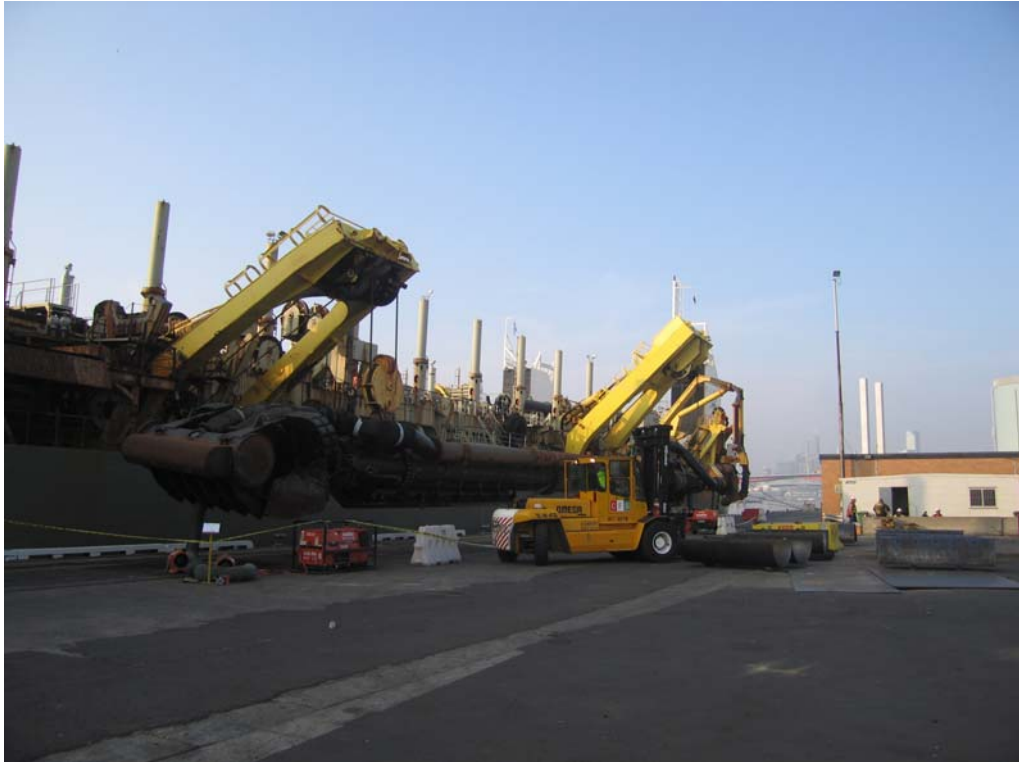
Figure 1: TSHD “Queen of the Netherlands” starboard suction pipe and draghead ready for inspection on 3/6/08
