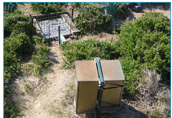
Photo: The weighbridge and data recording device
